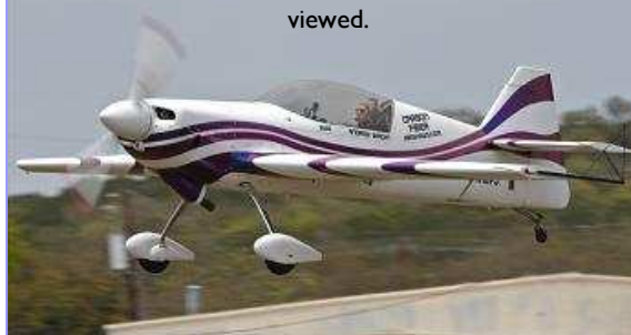
Giles 202 aerobatic aircraft. The chromatic paint changes color according to the angle from which it is viewed.
