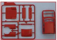
The truck body/box is five pieces; floor with inner fenders, outer fenders, front and tailgate. There is a roll bar in each kit, although if you use the gunner seat with the ZPU-1, the roll bar must be left off.
