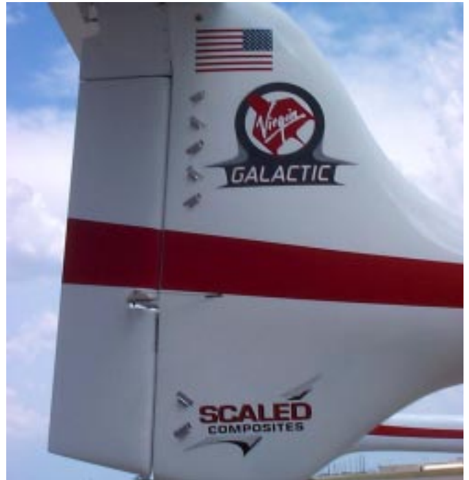
Vertical Fin/Rudder (note added-on airflow fences, simply bent aluminum sheet taped on both inner and outer surfaces with aluminum tape!)
