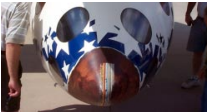
Nose with ablative material (the stripes are test strips that burn away at different temperatures).
