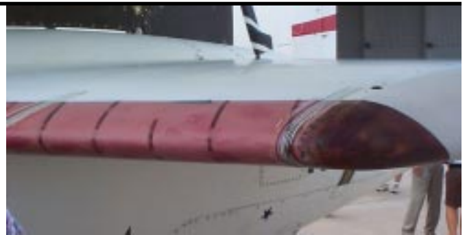
Wingtip with ablative material
