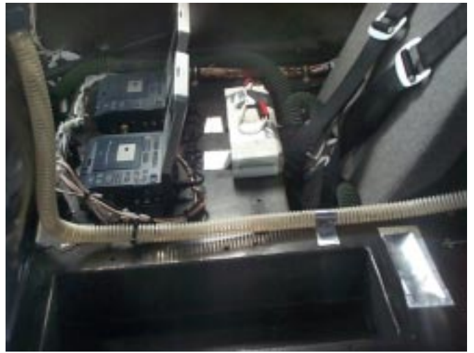
Right side “passenger” seat in SS-1 with ballast to represent occupant and recording instrumentation
