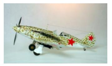
Looking at the finished product, the green should probably be greener, but I think I got what I was after. Final weathering involved exhaust and gun blast staining with pastels and mud staining on the undersides of the wings and tail surfaces as these units operated in some rough conditions. When weathering, bear in mind that this is a metal and wood airframe, so no paint chips on the outer wings and rear fuselage.
