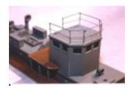
boat with tissue soaked in diluted white glue. This was later painted flat white. I then went to work on the bridge. I added windows all around by cementing thin clear plastic packaging material to the insides with Testors clear parts cement. Very handy stuff!
