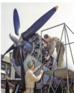
Center left and right: Two additional vintage color photographs of mechanics working on the huge Pratt & Whitney radial provide a good look at its details. Note the rounded conical shape of the reduction gear housing with the magneto on top of it. This early Thunderbolt has the original Curtiss Electric propeller installed. (Both, Bell Collection)
