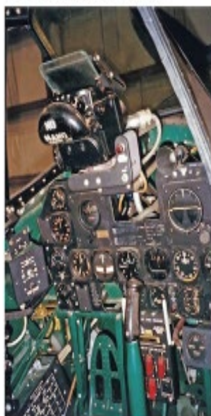
Above: The Yanks Air Museum in Chino, California, has a beautifully restored P-47M-1-RE. The original K-14 reflector gunsight was replaced by the Mk. VII gunsight with its rectangular reflecting glass beginning with the P-47D-40-RA, and the Mk. VII remained the gunsight in the P-47M. (Kinzey)
