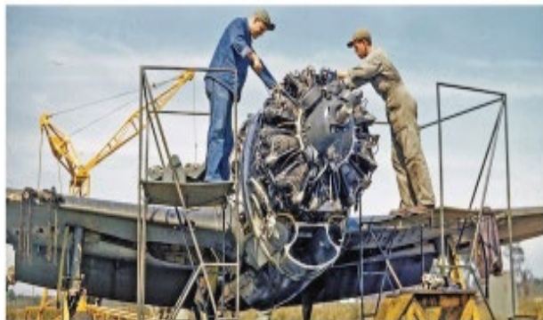
All production variants of the Thunderbolt were powered by the large Pratt & Whitney R-2800 Double Wasp, twin-row, eighteen-cylinder, air cooled, radial engine. The R-2800-21 engine was installed in the P-47B, but improved and more powerful versions of the engine were used in later Thunderbolt variants. Here, two mechanics work on the R-2800 on an early P-47. (Bell Collection)
