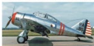
The P-35 was the first fighter aircraft developed by Seversky. It had semi-retractable landing gear, and it was powered by a Pratt & Whitney R-1830 radial engine that produced 850 horsepower. The P-35A in the photo at left is now on display at the National Museum of the U. S. Air Force. The sole XP-41 was a development of the P-35 that added a geared supercharger which increased the horsepower to 1,150. The design was sleeker than that of the P-35, and the landing gear was fully retractable. (Both, NMUSAF)
