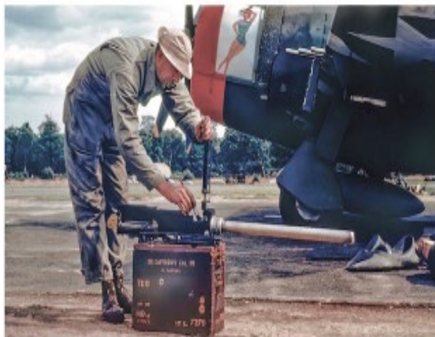
All production Thunderbolt variants had eight Browning .50-caliber machine guns as their internal armament. This made the P-47 the most heavily armed, single-engine fighter of World War II. Here, an armorer cleans one of the machine guns prior to installation in a P-47D. Note that the barrel is covered with a stainless steel tube. (Pier Collection)
