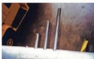
This top view illustrates how the barrels of the machine guns were staggered as they projected from the leading edge of the wing. Again, note the stainless steel tubes that cover the barrels. (Kinzey)
