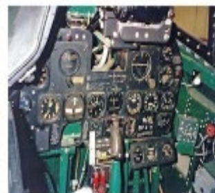
The instrument panel in the P-47M was very similar to that in late P-47Ds. The paint used in the cockpit matches what factory fresh Dull Dark Green would have looked like. Note the later style rudder pedal used in the P-47M. (Kinzey)
