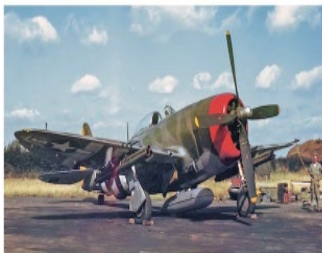
When used in the fighter-bomber role, rockets were an important addition to the Thunderbolt's arsenal of weapons. For P-47Ds during most of the war, this usually meant carrying M-10 "stove pipe" triple launch tubes for 4.5-inch rockets mounted under each wing between the landing gear and the wing pylons, as seen on this Thunderbolt assigned to the 56 th Fighter Group. Note the 150-gallon fuel tank below the fuselage. (G. Balzer Collection)
