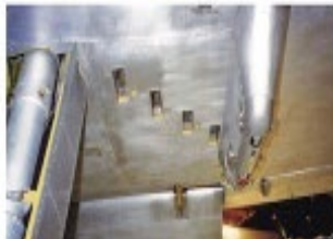
This top view illustrates how the barrels of the machine guns were staggered as they projected from the leading edge of the wing. Again, note the stainless steel tubes that cover the barrels. (Kinzey)
