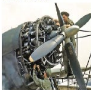
All production variants of the Thunderbolt were powered by the large Pratt & Whitney R-2800 Double Wasp, twin-row, eighteen-cylinder, air cooled, radial engine. The R-2800-21 engine was installed in the P-47B, but improved and more powerful versions of the engine were used in later Thunderbolt variants. Here, two mechanics work on the R-2800 on an early P-47. (Bell Collection)
