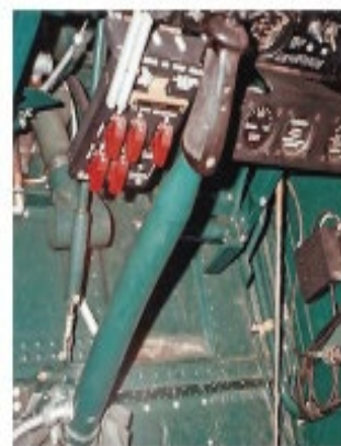
The instrument panel in the P-47M was very similar to that in late P-47Ds. The paint used in the cockpit matches what factory fresh Dull Dark Green would have looked like. Note the later style rudder pedal used in the P-47M. (Kinzey)
