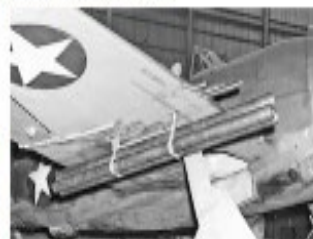
An overall view of a triple-tube launcher under the right wing shows how it was attached to the wing. (Bell Collection)
