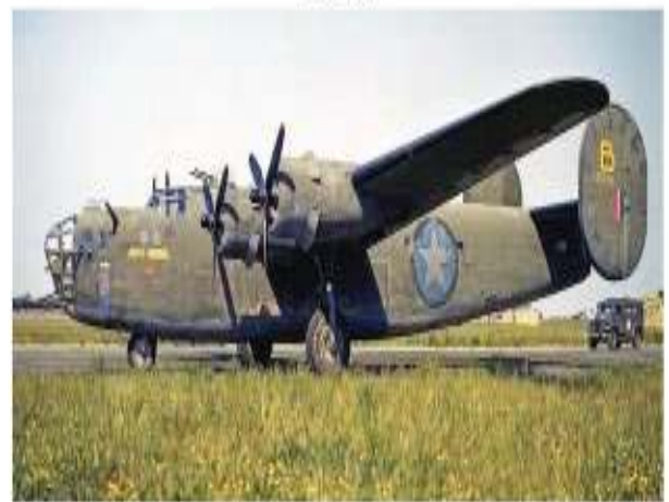
"JERK'S NATURAL" was an early production B-24D-1-CC. It was produced without the .50-caliber cheek guns in the nose, but by the time this photo was taken, the guns had been installed. The Liberator was assigned to 32nd Bomb Squadron, 80th Bomb Group, Eighth Air Force. When this photo was taken in England, it had already returned from its detachment to the Mediterranean Theater to participate in Operation Tidal Wave, the low level attack on the Ploesti oil fields. The aircraft was shot down on October 1, 1942, with the loss of nine of the ten crew members. (USAAF via Bell)
