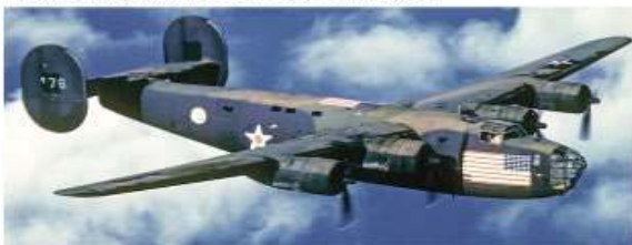
The RB-24As used by the U. S. Army Ferry Command were painted in the same brown and green camouflage used on British aircraft, but the vertical surfaces as well as the undersides were painted flat black. Large U. S. flags were painted on both sides of the nose and on top of the fuselage. (Piet Collection)
