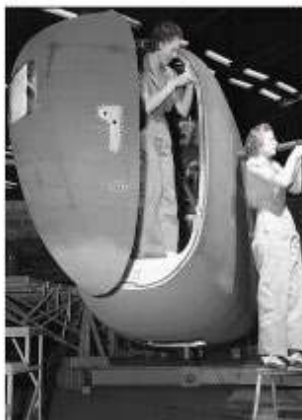
Employees on the C-87 production line work on the nose section. The photograph shows how the sheet metal nose of the Liberator Express was hinged on the right side to allow cargo loading. (Lloyd Collection)
