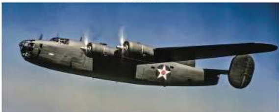
This in-flight photograph, taken at Wright Field, Ohio, in 1947, provides an excellent study of the features of the B-24A. These include the short nose with the framed glazing, the round engine nacelles, the silver discs on the front of the engines, and the location of some of the armament windows. Note also that the propellers are natural metal rather than being black. There were no turrets in any location on the aircraft. This B-24A is painted in the standard USAAF camouflage of Olive Drab over Neutral Gray. (Piet Collection)
