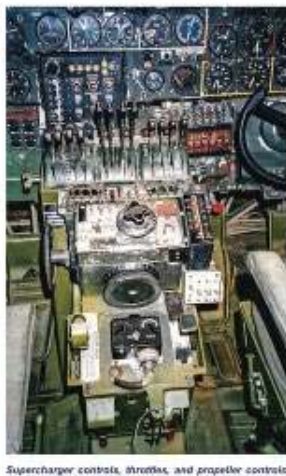
Supercharger controls, throttles, and propeller controls, as well as those for the intercom and cockpit heaters, were located on the pedestal between the two seats. Three control wheels are also visible. (Kinzey)
