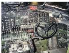
The cockpit in the Air Force Museum's B-24D remains virtually as it appeared when the aircraft was operational. Details of the pilot's instrument panel are shown in the photo at left. Features on the copilot's side of the instrument panel are illustrated in the photo at right. The engine instruments were the copilot's primary responsibility. Note the control yokes with the open top. (Both, Kinzey)
