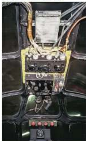
The overhead panel included the command receiver control box and the compass receiver control box. (Kinzey)
