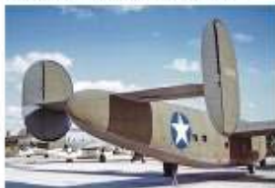
The unarmed C-87 had no tail turret. The aft fuselage was simply rounded off into an aerodynamic conical shape. The horizontal and vertical tail surfaces retained the same as they were on standard B-24s. (USAF via Bell)
