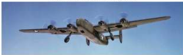
A C-87 Liberator Express takes off on a test flight from the Consolidated production plant at Fort Worth, Texas, in 1942. The C-87 was based on the B-24D airframe and was developed to carry passengers and cargo over long distances that were greater than those possible with the C-46 or C-47. (Library of Congress)
