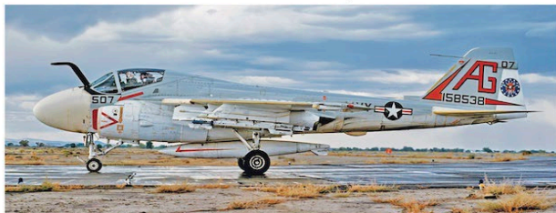
A-6E, BuNo. 158538, was photographed on a rainy September 28, 1976. This VA-65 Intruder is painted in the Gloss Light Gull Gray over Insignia White scheme. The radome and the engine inlet lip have an off-white appearance. The intake plate is painted Insignia Red, and the anti-glare panel and the refueling boom are painted flat black. The squadron markings on the vertical tail and the nameplate below the canopy are painted orange, outlined in black. In celebration of the country's 200th birthday, a bicentennial decal has been applied to the rudder. (Grove)
