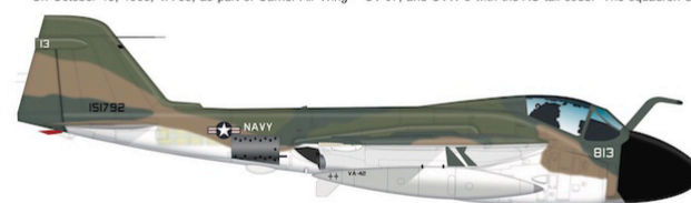
VA-85 experimented with various camouflage schemes during its 1965-66 deployment to Vietnam aboard USS KITTY HAWK, CVA-63. This A-6A, BuNo. 151792, was painted in a scheme similar to the Air Force A-6A camouflage scheme. The aircraft had neither a tail code nor the various warning and rescue markings, while NAVY and the modex on the nose and tail were painted white. The aircraft had small tri-colored national insignia on the aft fuselage and wings. Note the borrowed external fuel tank. (Roszak)
