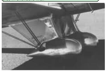
The original STA featured the Menasco engine and main landing gear and wheels fully enclosed in streamlined fairings, sometimes referred to as wheel pants. It had single-panel, curved plexiglass windshields. The XPT-16, YPT-16, and PT-16 all followed this configuration. Eventually, all but one of the 15 examples of the PT-16 series were adapted to the Kinner R-440 five-cylinder radial and re-designated PT-16A.
