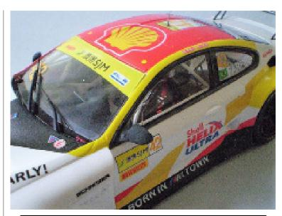
I went with a hybrid approach with the wiper blades on my model. I used the plastic wiper arms and replaced the blades with the photo etched version.
