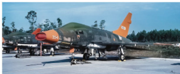
This well worn QF-100C, S/W 55-3557, was photographed at Tyndall AFB in October 1958. Of particular interest here are the pointed out canopy, the flame predictors, or "wing tip burners" used to draw heat seeking missiles out away from the aircraft's fuselage and therefore prolong its useful service life, and the red star insignia added to the paint patch used to cover the national insignia. (Leader)
