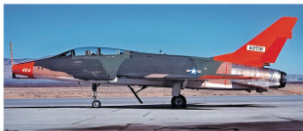
Like F-100Ds, some F-100Fs were converted to QF-100Fs and used as drones and drone controllers after being retired from ANG service. S/W 55-3791 is seen here after its conversion for the drone program. Note the lack of an ejection seat in the rear cockpit. (Grove)
