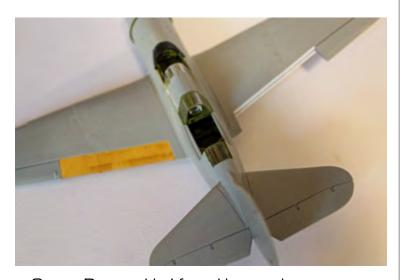
On my Dragon kit, I found it eased assembly considerably to cement strips of .030 inch square styrene strip to the rear edges of the wing halves to give a ledge to support the brass replacement flaps.
