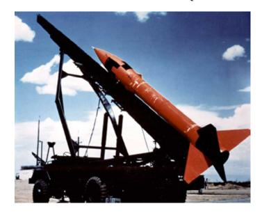
The MGR-1A was lower power (range 3-15 miles), larger fins, and weaker spin thrusters. It was launched from M289 truck, with a long rail which stretched beyond the length of the truck and had a brace underneath.
