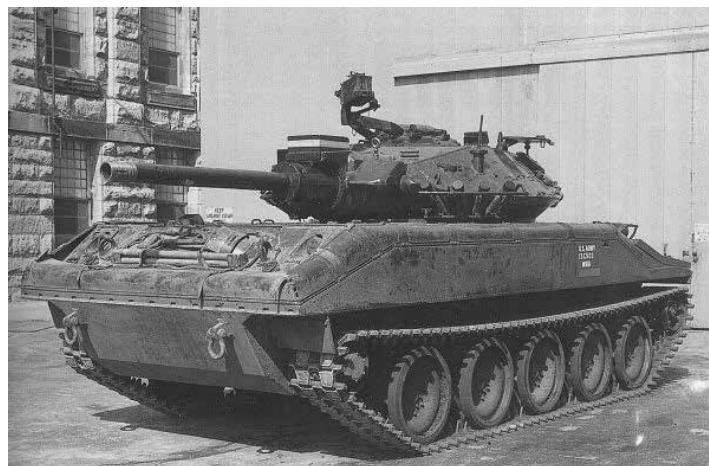
M551 fitted with 105 mm gun
