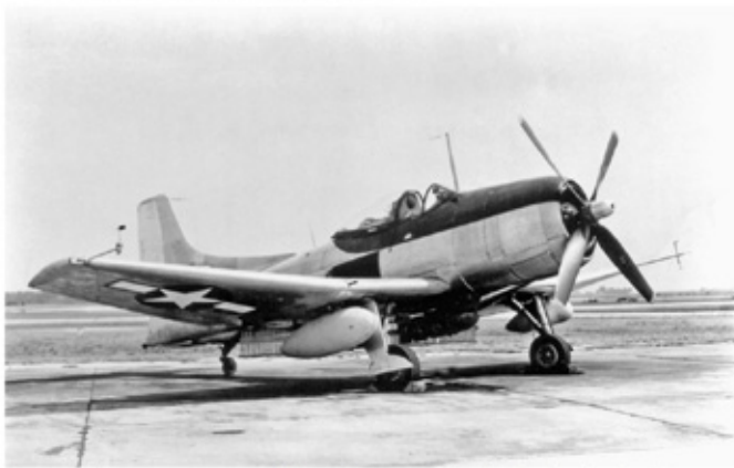
The Kaiser-Fleetwings XBTk-1 was one of the single-seat torpedo bombers developed under the new Navy design criteria specifying a single aircraft type to replace both dive and torpedo bombers. Note the external fuel tanks under the wings and the bomb under the fuselage. (National Archives)
