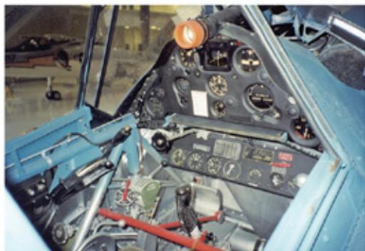
The National Naval Aviation Museum at Pensacola, Florida, has restored an SB2U-2 Vindicator to original condition. Details of the pilot's instrument panel are revealed in this view. (Kinzey)
