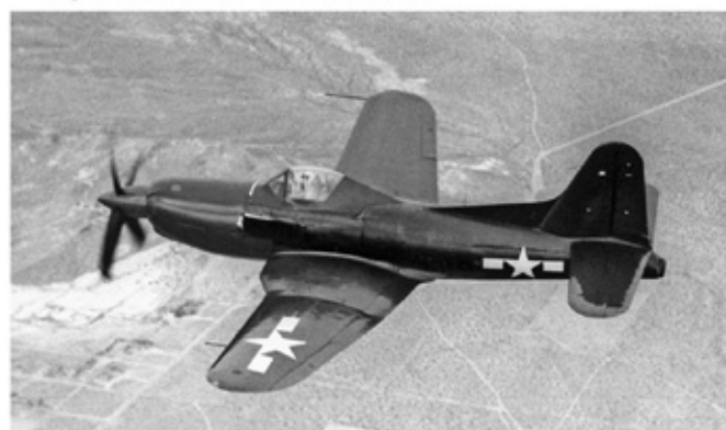
The XF2R Dark Shark was a further development of the FR-1 Fireball. It replaced the Wright radial engine with a General Electric XT-31-GE-2 turboprop powerplant mounted inside an extended nose. (NNAM)
