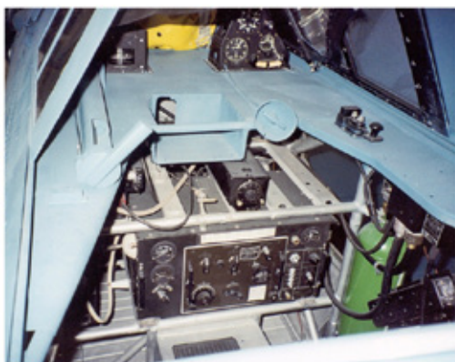
Some of the radio gear in the rear cockpit is shown here. Note the key for sending Morse code on the deck to the right. The green bottle contained breathing oxygen for the radio operator/gunner. (Kinzey)
