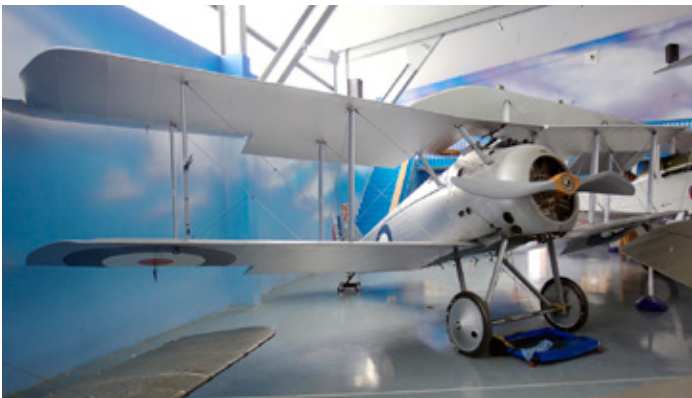
Sopwith 7F.1 Snipe replica built in 2013 by TAVL, cn: 114, is registered as ZK-SBY. Powered by a 230hp Bentley BR2 rotary engine, the aircraft is depicted as 'E7643' of the Royal Flying Corps.
