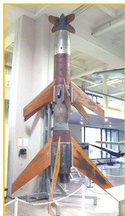
Here is the real thing. The wings/guide vanes were made of plywood!
