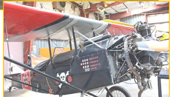
1979 Pietenpol Air Camper, RN1, with a five-cylinder Lambert radial engine.
