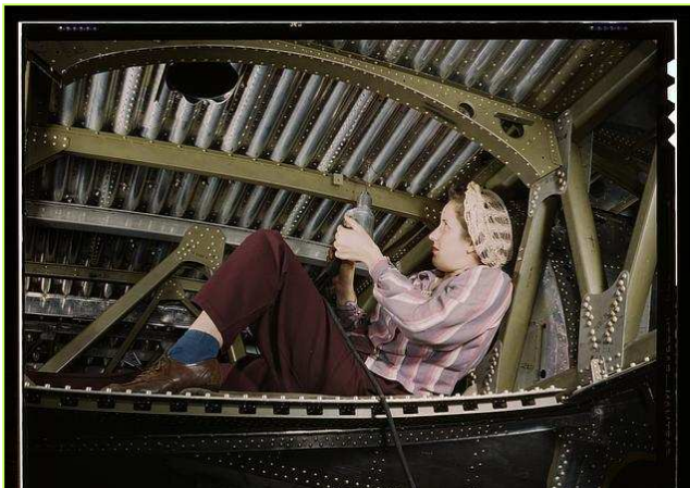
An A-20 bomber being riveted by a woman worker at the Douglas Aircraft Company plant at Long Beach, Calif.
