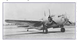
mid-wing monoplane with a narrow fuselage enclosing four crew positions and an internal bomb bay. It had a retract-
