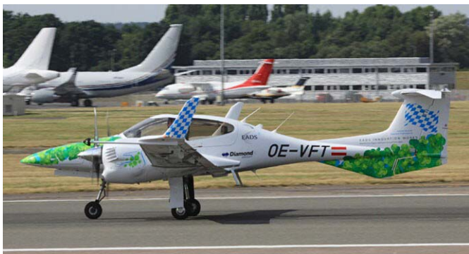
This DA-42 deserved to be the "greenest" aircraft at this year's Farnborough air show. One of its engines is powered by diesel and the other by specially grown algae bio-fuel. Manufactured by EADS, parent company of Airbus, it claims the new alternative fuel is 10% more efficient than diesel and carbon-neutral (CO 2 released by fuel burn is less than that consumed by the algae during growth).
