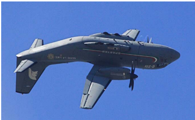
C-27J Spartan performing a "whale breaching" maneuver. Utilizing the engines of a C-130J Super Hercules, the C-27J is an advanced derivative of Alenia Aeronautica's G.222. The aircraft has been selected as the Joint Cargo Aircraft (JCA) for the US military.
