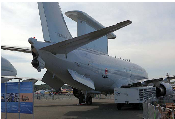
Boeing 737 AEW&C in Turkish Air Force service. Roughly half the weight and engine size of a 707 based E-3, it features an electronic scanning antenna instead of a conventional rotating radar dome. Designed for RAAF under "Project Wedgetail," it is currently been used also by ROK Air Force.
