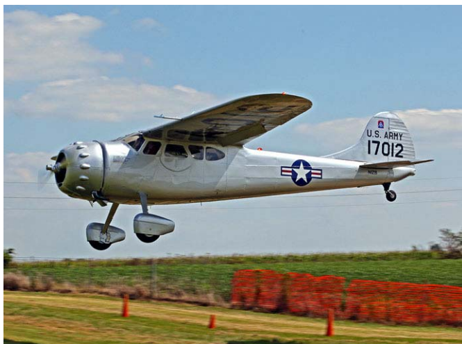
This Cessna LC-126C (N1ZB) is the military version of the 195 Businessliner. The 190/195 were Cessna's only post-war radial engined aircraft, according to the entry in Wikipedia.
