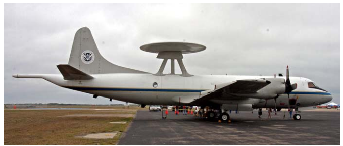
Real life kitbashing: an E-2 Hawkeye dish on a P-3 Orion! Department of Homeland Security has eight of these AEWs for border patrol and anti-drug duties.
