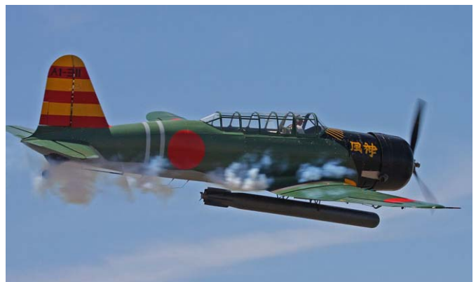
Formerly a Canadian Air Force Harvard/Texas, it was converted to look like a IJN Kate torpedo bomber for the Tora, Tora, Tora Reenactment.
