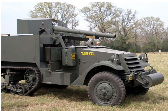
75mm Gun Motor Carriage M3 — US first attempt of a tank destroyer by mounting an American version of a WWI French gun on the M3 halftrack. According to the announcer, this vehicle is only example in running condition left in the world.
