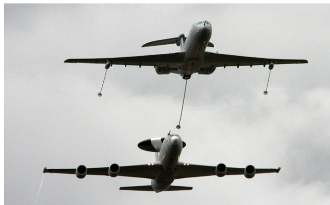
BAC VC-10 C.1K simulates low-level aerial refueling of Boeing AEW.1 during RAF 90 th Anniversary fly-by for The Queen.
