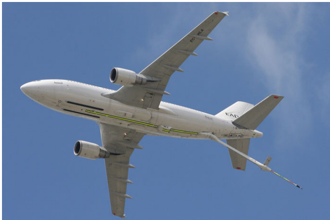
Airbus A310 MRRT, EC-HLA, used in the development of the refuelling boom for EADS tanker aircraft, including the KC-45A.
