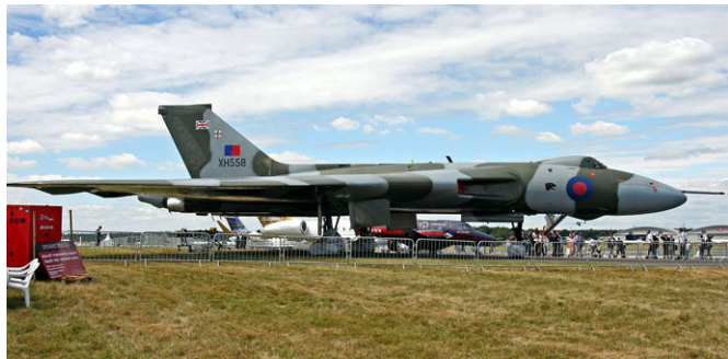
Avro Vulcan G-VLCN (ex XH558), recently restored to flying status, with about 5 tons less wiring than the original aircraft.
