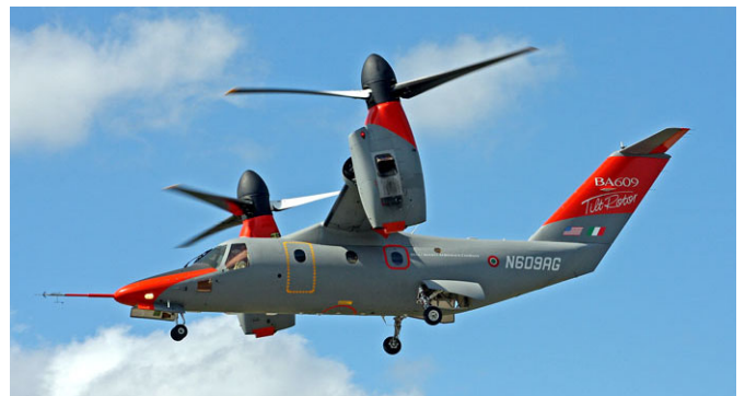
Bell-Agusta BA.609 tilt rotor prototype, N609AG, demonstrated flying forward, backward, and hovering.
