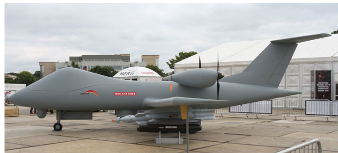
BAe Mantis UAV. Twin-engine mid- to high-altitude Intelligence, Surveillance, Target Acquisition, & Reconnaissance vehicle. Its first flight is planned for 2009.
