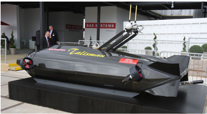
BAE Talisman. Unmanned underwater vehicle. Carbon fiber composite hull with four vectorable thruster pods.
