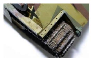
The tow cable was made per Tamiya's instructions using the kit supplied nylon thread. Accustomed to using aftermarket cables in the past, I gave up doing tow cable the "nylon" way a long time ago. But being lazy and stingy these days, I'll do anything to save a buck! After a bit of fidgeting and drilling on the boots of the cable, I got it to work, and it didn't look too bad after all.
