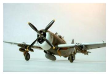
There were other touches that I won't detail here, such as using CA to replace the wing-tip formation lights, and rebuilding the sway braces—that I broke off—for the centerline tank.
